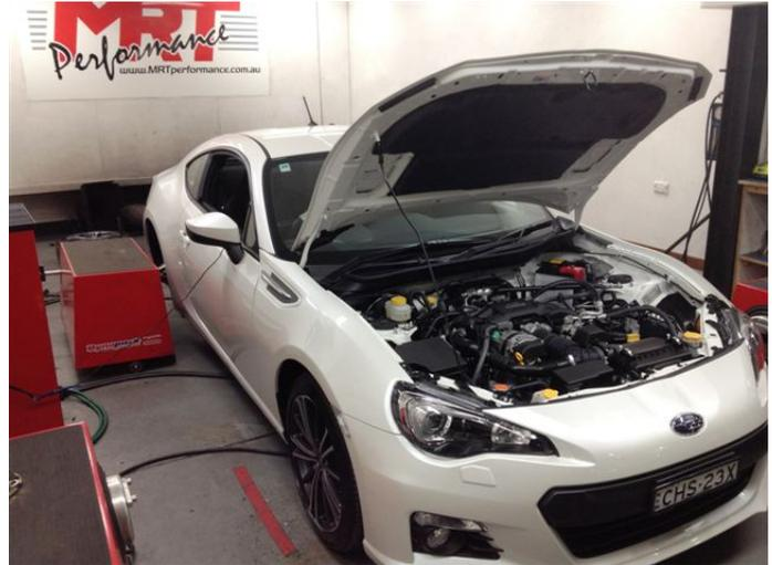
Before we get into the results, as an interesting side note the first 20km or so travelled in the car were on our dyno being run in and tested. The car then had a further 650km or so of road use stacked on with suspension and brake development being undertaken, before making its way back to the dyno for final testing and engine management system calibration development.
